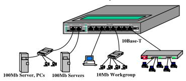
Figure 2.4c: Using a Magnum 528 Switch, 100Mb servers and users are added to an existing 10Mb network
